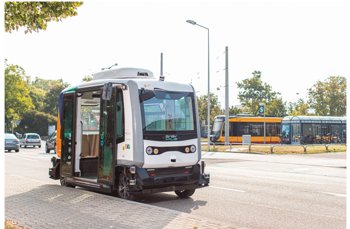
Fig. 1: The EVA shuttles Ella, Vera, and Anna have been deployed in Karlsruhe Dammerstock-Weiherfeld in the Test Area Autonomous Driving Baden-Württemberg. The shuttles choose their movement freely between road boundaries.
