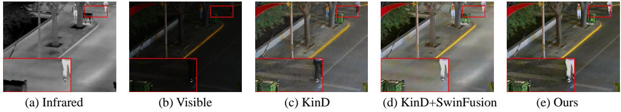
FIGURE 1 Nighttime visible image enhancement result and corresponding infrared image fusion results. In comparison to the fusion output achieved by SwinFusion (J. Ma et al., 2022) on the enhanced version by KinD (Y. Zhang et al., 2019), our proposed method effectively preserves a greater extent of enhanced details and yields a more favorable visual perception while the SOTA method hides the texture details again. To facilitate a more comprehensive comparison, regions exhibiting abundant textures were magnified within the red boxes.
