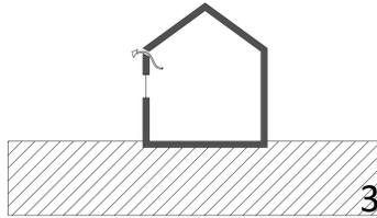
important to lower the dispersion surface, this condition can be satisfied by also creating a building that is in part buried (fig.1 vs fig.2), which reduces the area that loses heat to the external air (soil has a constant temperature of 12°C, while air can reach -10°C).
