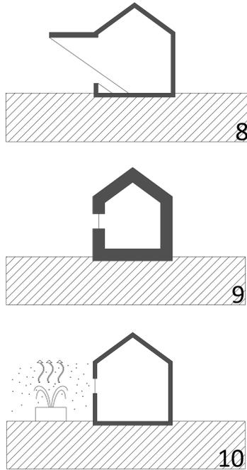
materials, which store heat during the day avoiding overheating and, with an effective ventilation of the indoor ambient, release it during night (fig.9).
