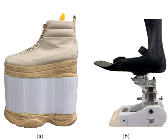
Fig. 6: (a) Leg length discrepancy shoe and, (b) 3-DOF prosthetic with a mounted socket simulator used for the gait trials.
