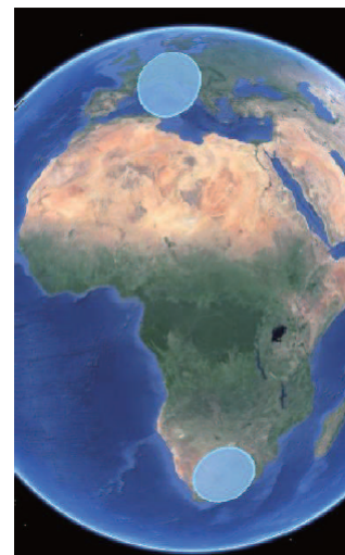
Fig. 1. Footprints of a telecom compatible geosynchronous SAR [11].
