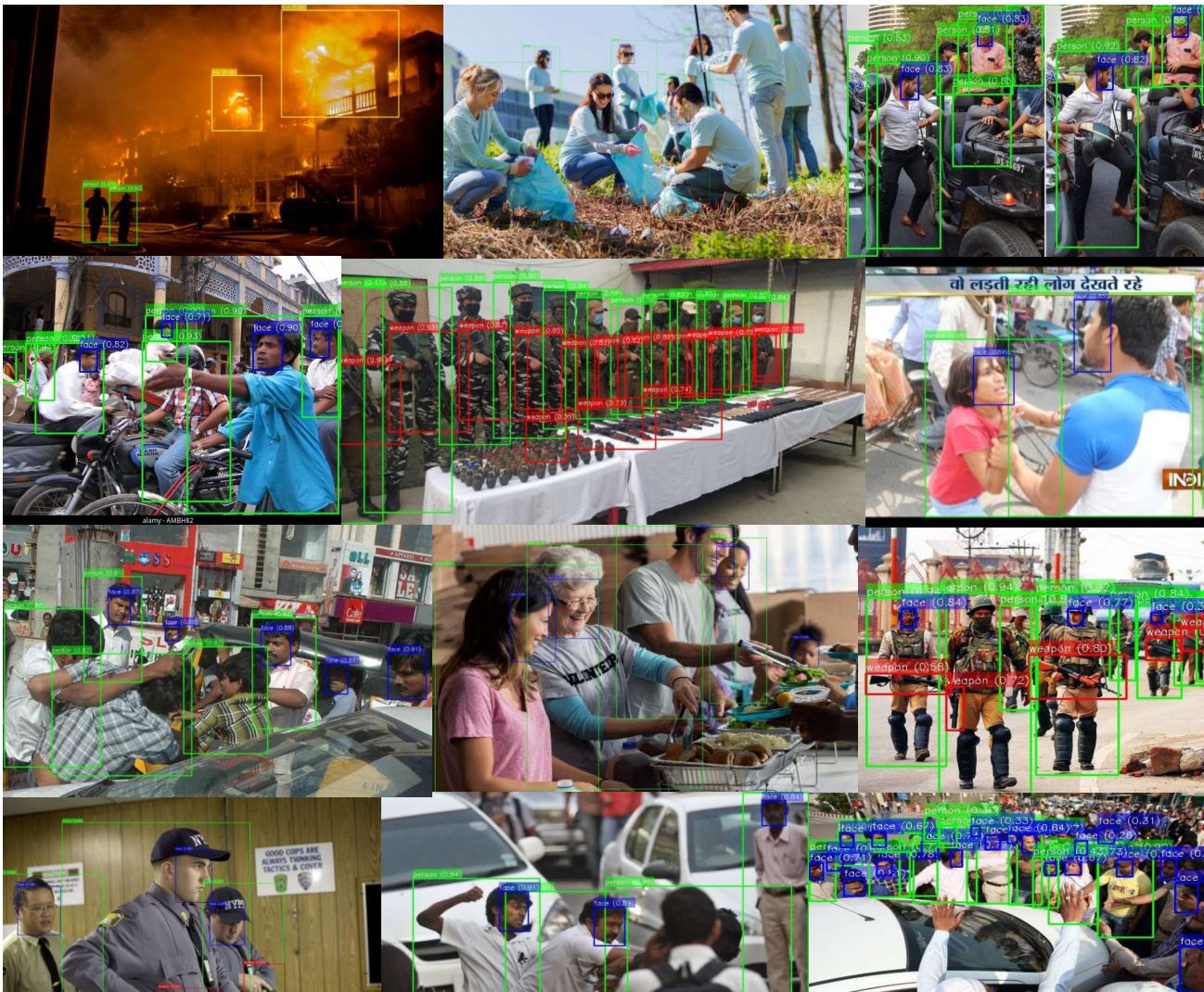
Fig. 10. Some samples from IITD-USE evaluated through the SOD model: green color bounding boxes represent the Person , blue color bounding boxes highlight the detected Face , red color bounding boxes represent Weapons , while yellow color bounding boxes highlight Fire .
