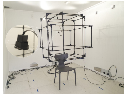
Fig. 4. DASS's coils installed in room 2. Each pair of Helmholtz coils comprises square coils of 1\text{ m} \times 1\text{ m} dimension located 0.5\text{ m} apart and positioned in the three orthogonal planes. The QuSpin Gen-2 OPM, that is the internal reference sensor, shown in the inset.
