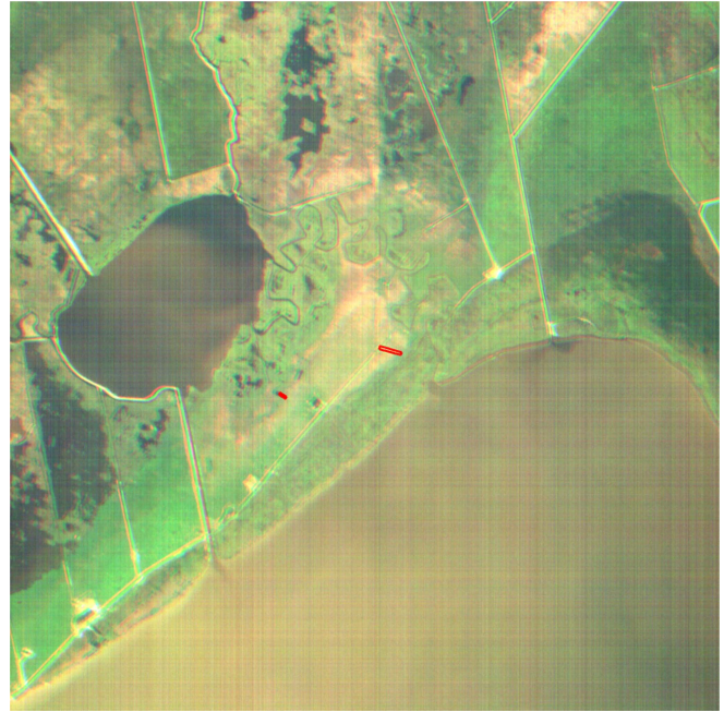
Fig. 13. Crop of the first image (of Galveston, Texas) analysed using a neural network on board with results relayed over ISL. Red boxes indicate the ship detections received on ground. Two false positive detections are visible. Since this is level 0 data with enhanced contrast for visualisation purposes, some image artefacts such as band-misalignment and striping are visible.
