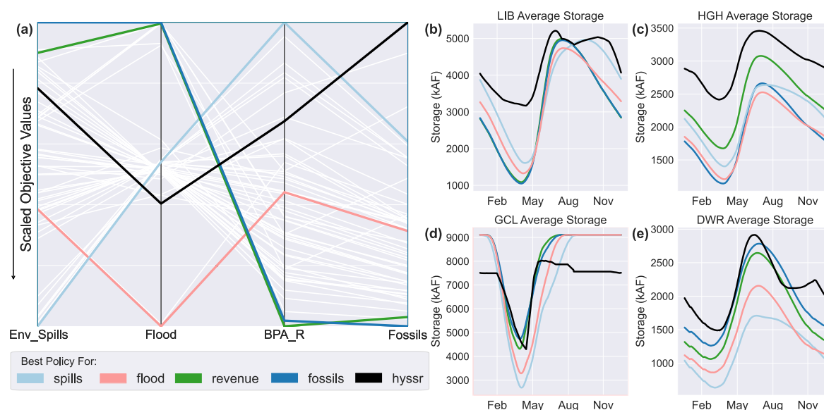
Figure 6. (a) Policies that perform best on each of the four objectives and HYSSR. (b-e) Average daily reservoir storage levels of the four optimized policies that are best on each objective and HYSSR at (b) Libby, (c), Hungry Horse, (d) Grand Coulee and (e) Dworshak.
