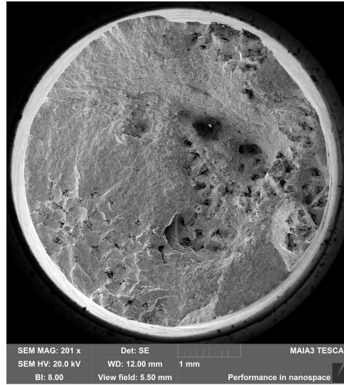
Figure 7: An example of a SEM image of one of the specimens from batch P3 which was dismissed from the analyses of this study due to high porosity which resulted in relatively low fatigue life.
