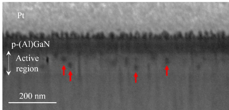
**Fig 1** SEM image from FIB cut of BAlGaN LED material. Voids can be seen in the active region of the LED (some of them are highlighted by the red arrows), showing an effect of boron.
