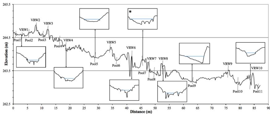
Figure 2. Reach profile from upstream (left) to downstream (right) with representative pool (above profile) and rock weir (below profile) cross-sections. The asterisk in the Pool 7 cross-section indicates the stilling welling location. Vertical exaggeration is 0.08 m.
