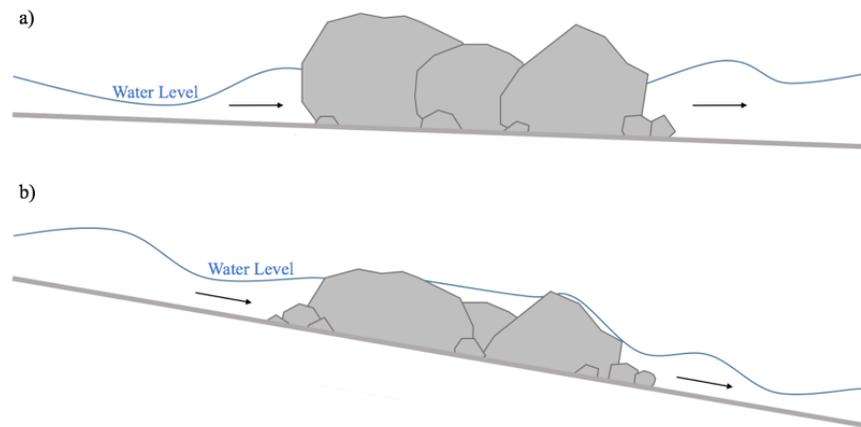
Figure 4. Profile schematics of a low gradient rock weir (a) and high gradient rock weir (b). The difference in gradient depicts how embeddedness changes depending on how gentle or steep the channel bed is. A greater level of embeddedness provides upstream and downstream connectivity without obstructions to the flow path (b).
