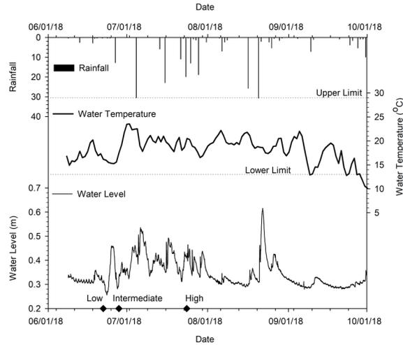
Figure 1. Daily rainfall, daily water temperature, and hourly water level along the study reach. Upper and lower temperature limits for fish species local to Weslie Creek are labeled on the water temperature graph (LSRCA, 2000; Eakins, 2018). Field assessment days are shown with diamonds along the lower x-axis.
