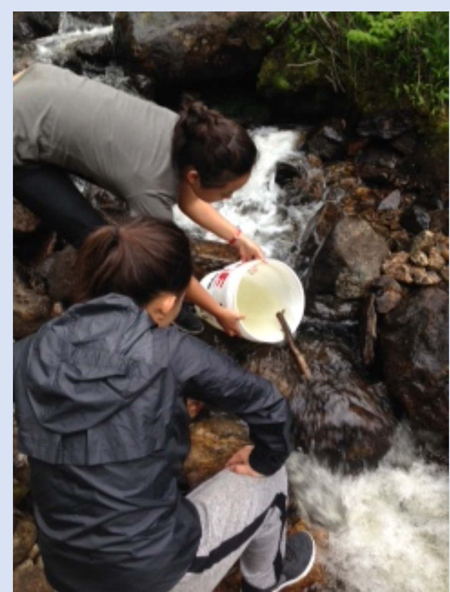
Fig 5. Students injecting conservative salt tracer for discharge computation.
